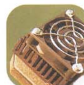
Temperature control: Peltier heat transfer controller
